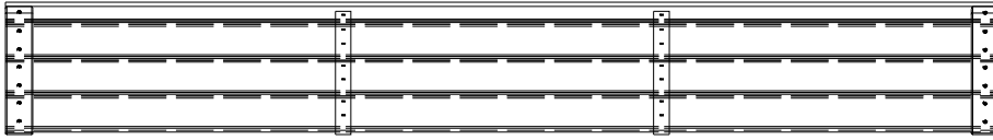
RP01 | ROOF PANEL - W2A02182 (x1) | 1/16"x1/16"x1/16" (40x287x2165)
