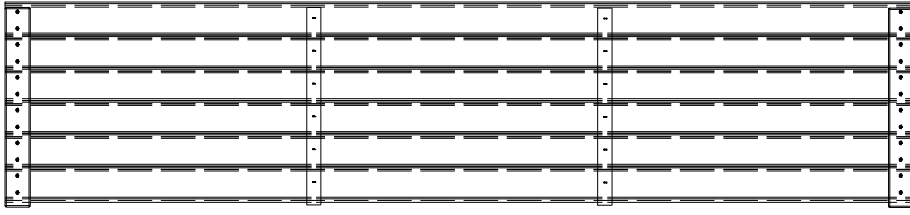
RP02 | ROOF PANEL - W2A020184 (x1) | 1 9/16"x19 1/4"x85 3/16" (40x488x2165)
